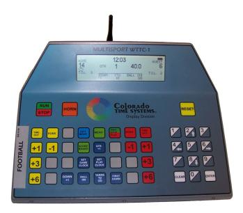
The wireless tabletop controller features an operating distance up to 1,000 ft., buttons with tactile dome feedback, and a large transflective LCD screen that is easily readable in all environments from darkness to bright sunlight. The controller includes a built-in real time clock to keep time of day.
