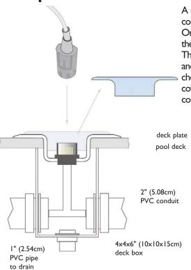
A military connector with gold-plated connections is mounted in the pool deck. One short cable runs from this deck plate to the connection hub under the starting block. This system provides greater convenience and less possibility of corrosion from pool chemicals and water. The connector is covered when not in use to prevent corrosive build-up.
